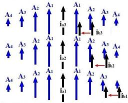
Magnetic coupling force works between ia and ib through vector potential A
